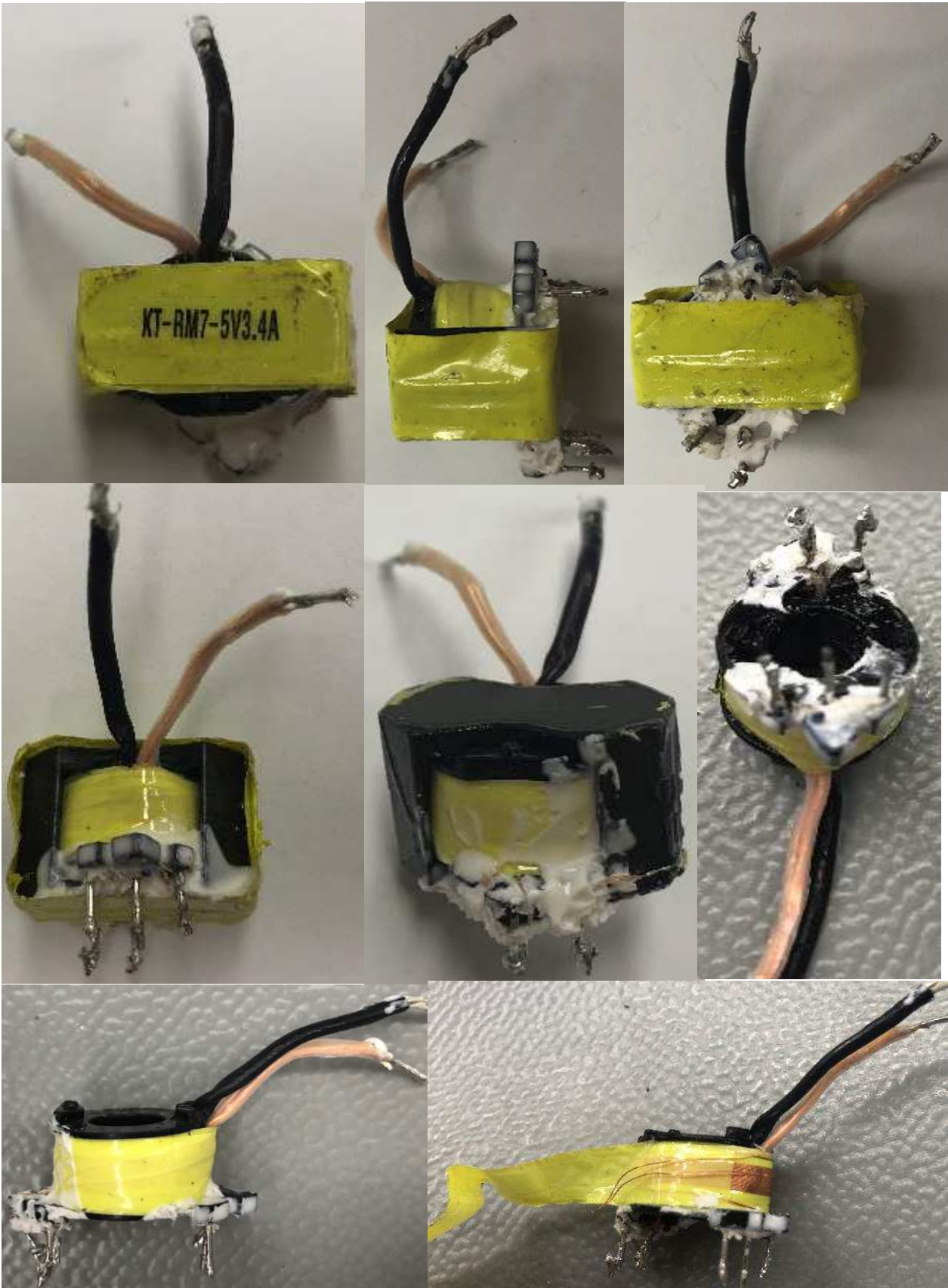
Photo 11 - Transformer for class 2 power unit KT-CU2301-5V3.4A
