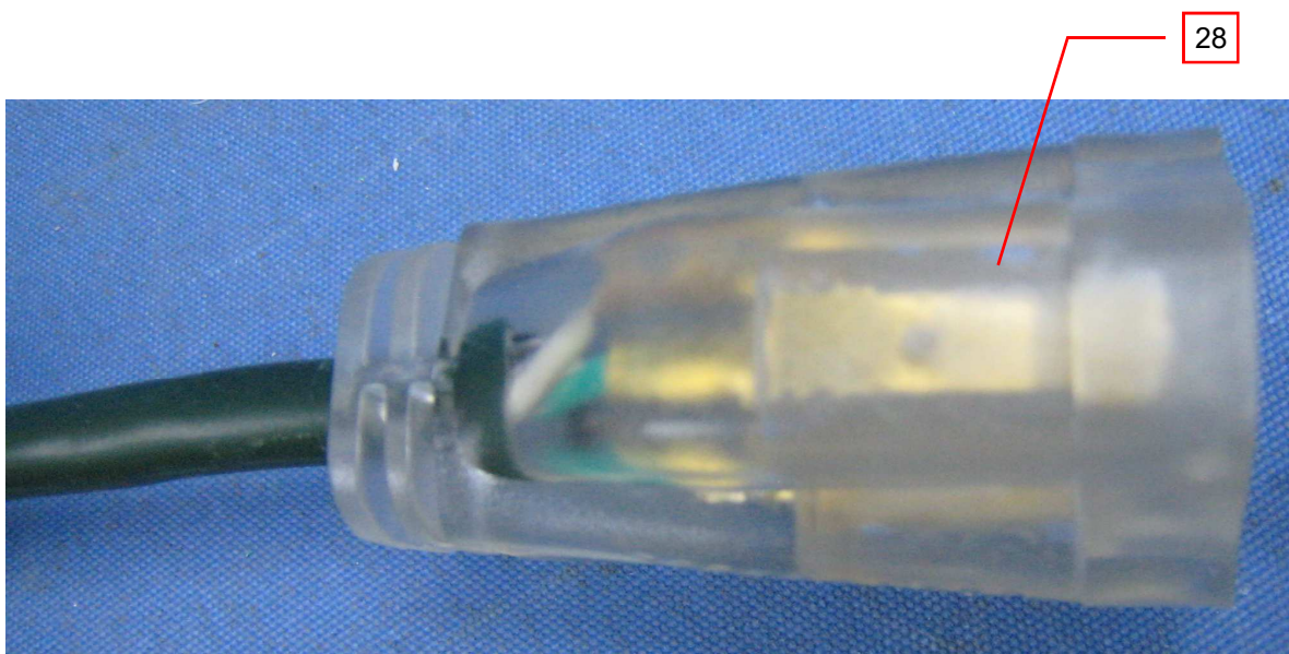
Photo 18 - Overall view of cord connector KT101 (with alternative insert)
