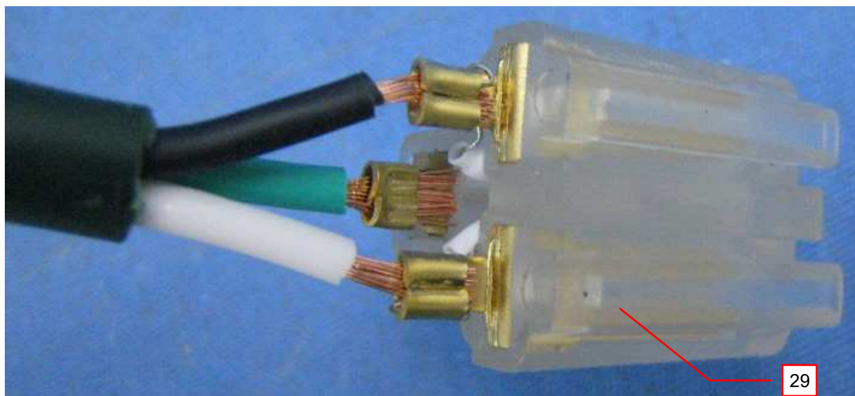
Photo 22 -Alternative insert for cord connector KT101
