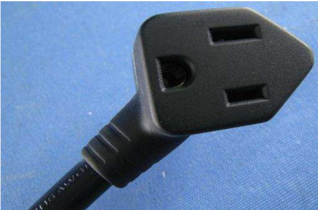
Photo 11 - Overall view of current tap part of 40106A
